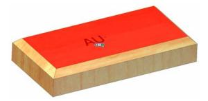
O 37. Autoproject edges can cause difficulty in selecting text sketches, but you can use the Select Other tool to get the text.
