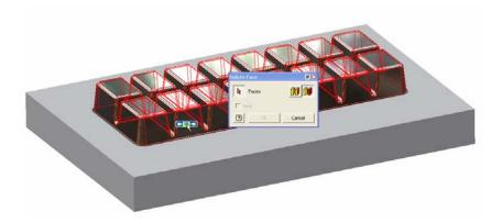
O 69. Use **Derived Components** to create tooling dependencies. If the part changes the tool changes. Use the **Delete Faces** with the **Lump or Void** option to delete an internal void.
