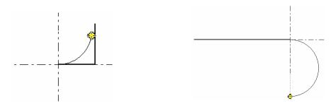
O 28. You can use the shortcut **L** to create a **Line** and an arc from a line endpoint by click dragging from the endpoint while in the line command.
