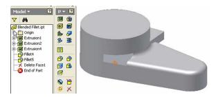
O 62. If you start working with surfaces be sure you understand when you have a surface and when you have a solid. (A surface feature will be translucent or a surface created from a solid by the Delete Face tool will show at the top of the browser as a surface icon. If you use the Delete Face tool solid options will be disabled until you stitch your surfaces back to a solid.)
