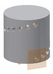
O 60. The **Coil** command in Inventor 11 now allows creation of a surface. The edge of the coil surface can be used for a pattern curve.
